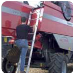
Easy access via removable ladder to the engine bay and grain tank
