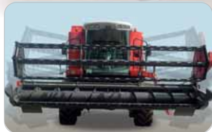
All Activa combines have the option of being fitted with an Auto Level table, which is able to follow changes of up to 8% in ground contours
