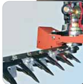
All Activa combines have the option of being fitted with an Auto Level table, which is able to follow changes of up to 8% in ground contours
