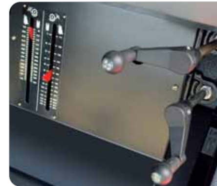
Two levers adjust concave clearance front and back
