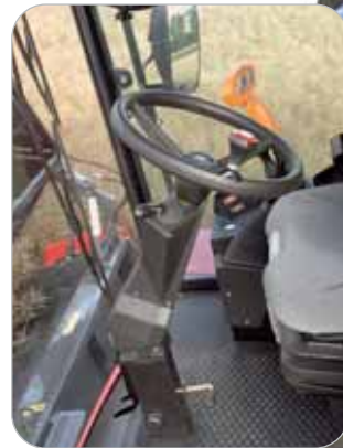
The steering column adapts to the operator's driving position
