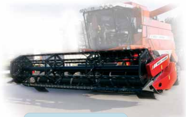
All Activa combines have the option of being fitted with an Auto Level table, which is able to follow changes of up to 8% in ground contours
