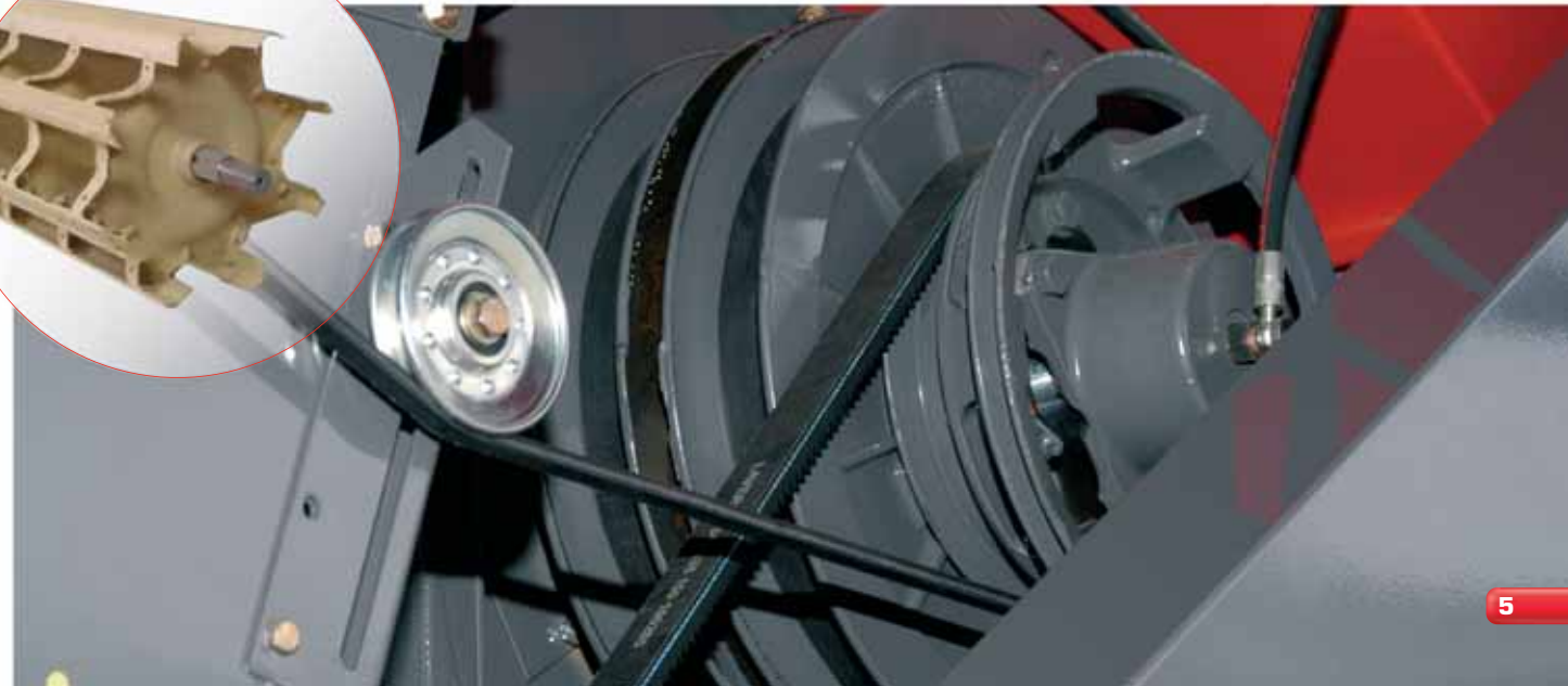
Cylinder speed remains constant due to significant wrapping of the variator pulleys, so optimising machine performance
