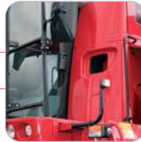
A wide inspection hatch, accessible from cab platform, allows the driver to take a grain sample to check the quality
