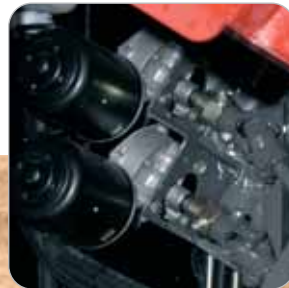
Two electric motor controls from the cab adjust the concave clearance
