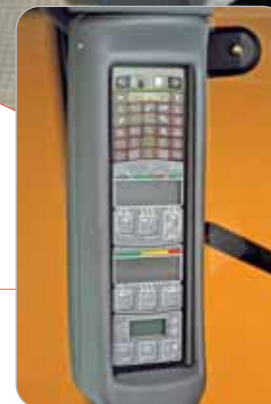
The Agritronicplus unit allows the operator to monitor correct machine operation, shaft speeds, machine performance and cutting height
