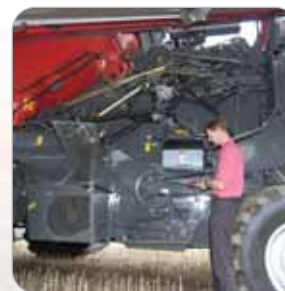
Hinged side panels give clear access to main drives and belts
