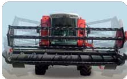
All Beta combines are fitted with an Auto Level table as standard, which is able to follow changes of up to 8% in ground contours
