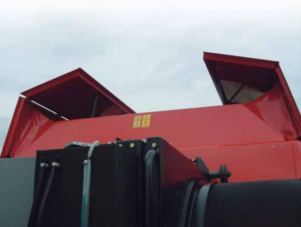
The grain elevator augers and caps have "Hardox" hardened ends for maximum service life
