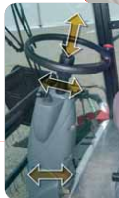
The steering column height and tilt adapts to the operator's driving position
