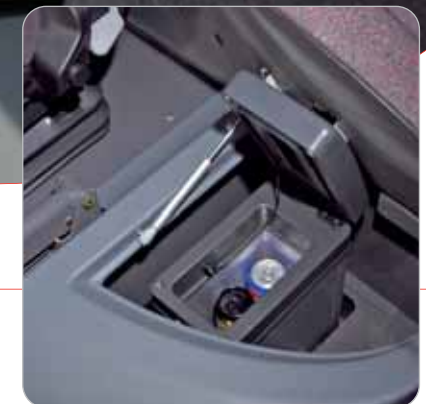
A large refrigerated compartment under the passenger seat can hold up to two 1.5 litre bottles
