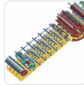
Powerfeed roller is located at the front of the main crop elevator
