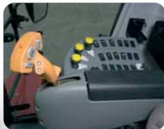
The hydrostatic control lever and all the combine controls are mounted on the right hand armrest
