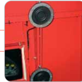
Two sensors monitor the grain level in the grain tank and alarms on the Agritronicplus monitor
