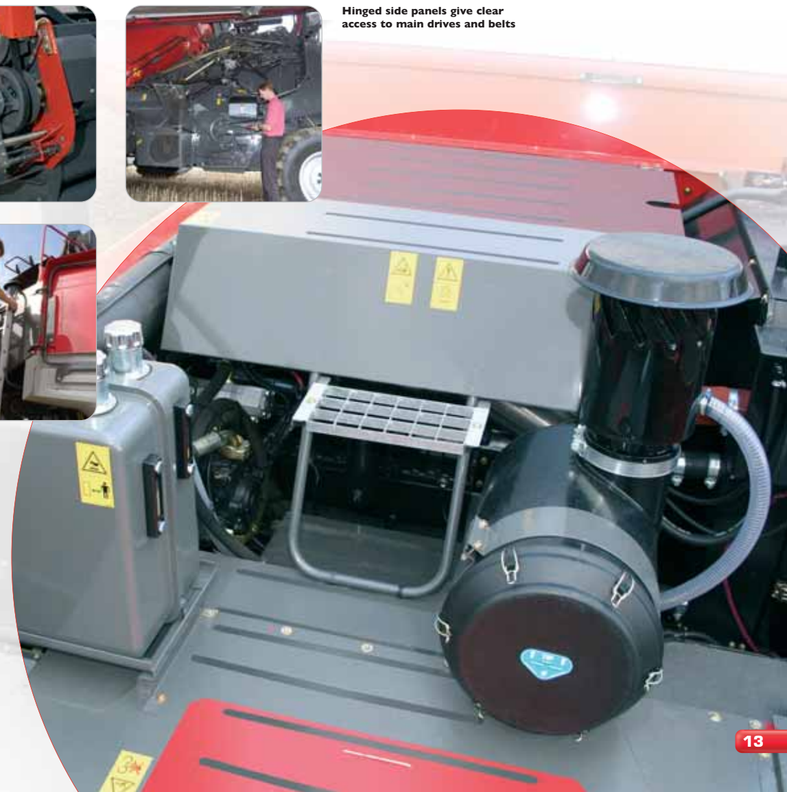
Easy access via removable ladder to the engine bay and grain tank
