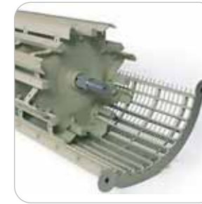
Differential wire spacing on concave
