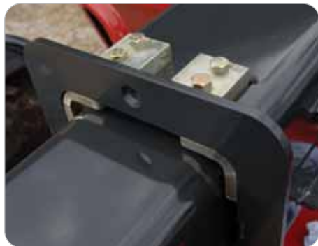
Below: Maintenance made easy - The boom is simple to remove for routine servicing of the wear pads
