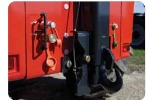
Above: Double-acting rear hydraulic outlets and a hydraulic trailer braking facility may be specified to accompany the optional hydraulic hitch
