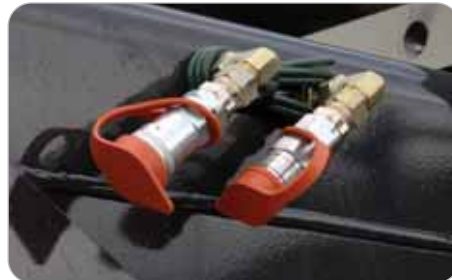
Above: Coupling and uncoupling of hydraulic attachments is quick and simple
