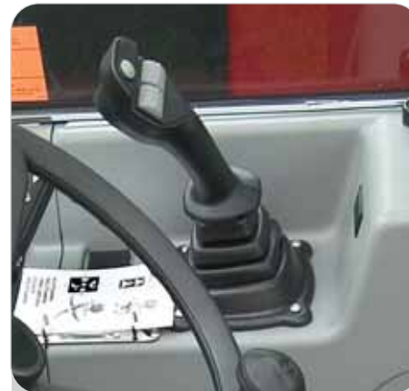
Our designers have made the features of the telescopic arm easy for you to control through a simple, multi-function joystick for the boom and attachments and a finger-tip lever for speed range and directional control
