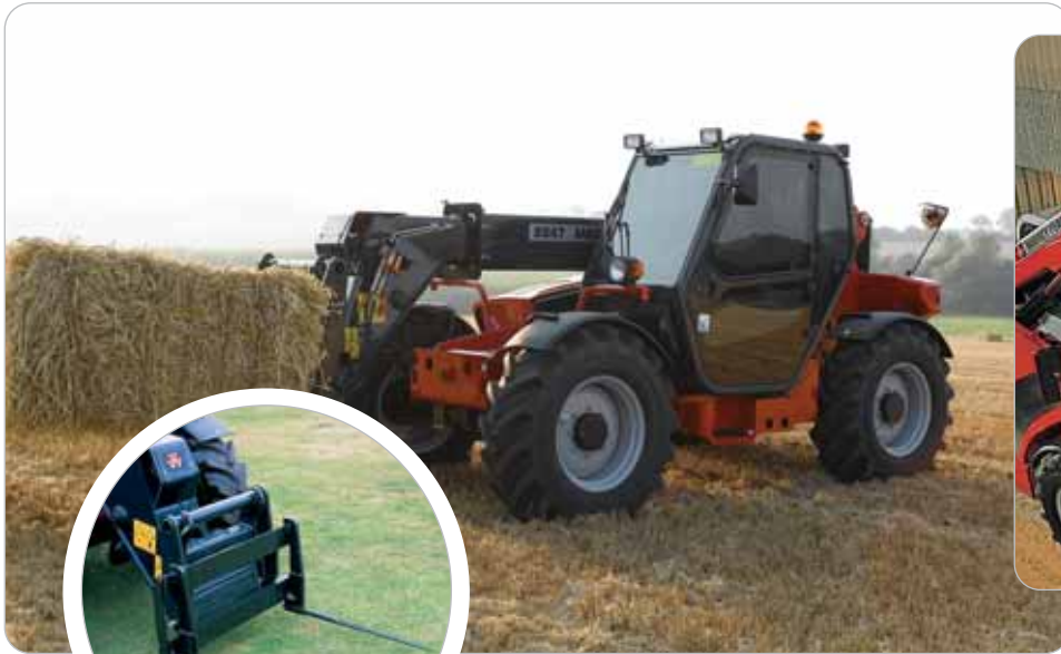
Bale spikes for precise bale handling
