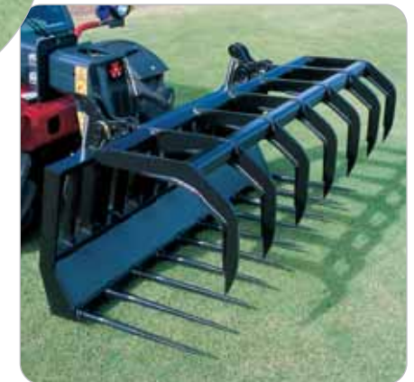
Grab and spike option for secure and easy carrying
