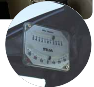
On the 89410L models with hydraulic frame levelling, an in-cab inclinometer indicates chassis-horizontality to aid safe operation
