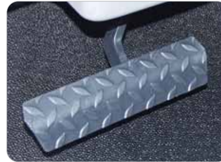
The inching pedal (above): initial movement of the brake pedal enables slow, controlled movement - even at full engine speed
