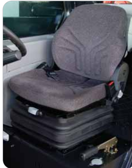
The pneumatic suspension seat is fully adjustable to suit the weight of the driver
