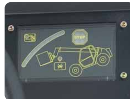
The dash-mounted overload indicator is clearly legible in all lighting conditions
